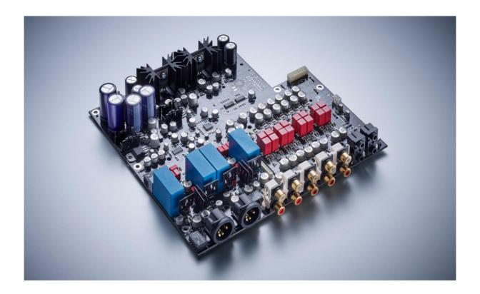
The multi-channel output stage is a scaled-down version of the stereo output stage, driven by a Crystal CS4382A multi-channel DSD DAC in conjunction with an analogue stage comprising Burr Brown OPA2134 OP-Amps, WIMA and NPO SMD capacitors and large MELF resistors.
